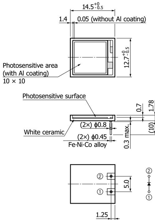
Note: Al thickness on photosensitive surface approx. 1  $\mu\text{m}$
