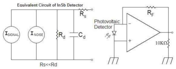
When background radiation shifts the operation curve by generating a constant output in the active element, the detector should be reversed-biased to bring it back to the optimum operating point: zero voltage.
