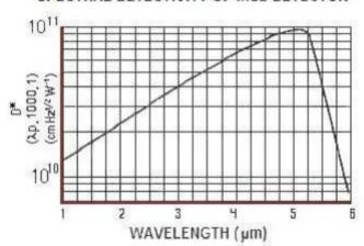
The photovoltaic effect is the generation of a potential across the p-n junction when radiation of the proper wavelength is incident upon it. When the photon flux irradiates the junction, electron-hole pairs are formed if the photon energy exceeds the forbidden gap energy.
