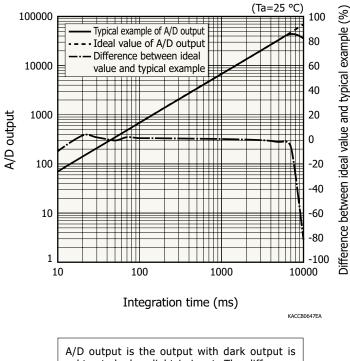
subtracted when light is input. The difference between the ideal value and typical example contains a measurement error. The smaller the A/ D output, the larger the measurement error.
