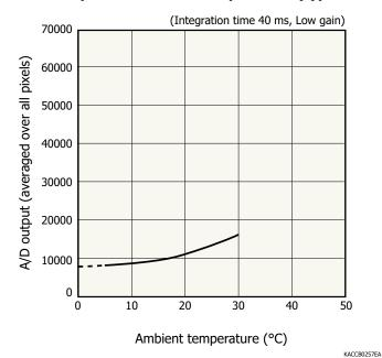
A/D output is the sum of the sensor and circuit offset outputs and the sensor dark output.
