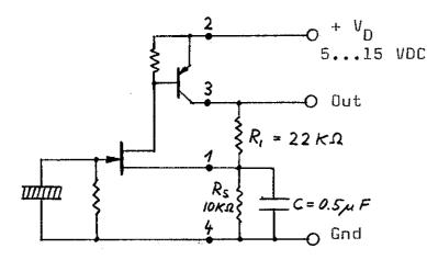
Open loop gain : 200 ... 400 Input stage is noise limiting. D\* performance remains unchanged in respect to unity gain circuit.
