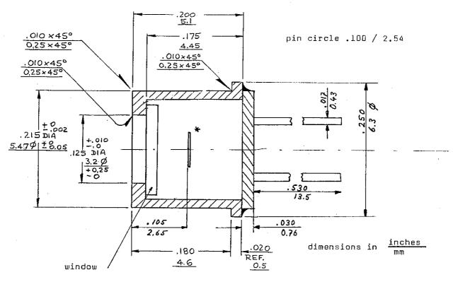
\* apparent position of sensing element
