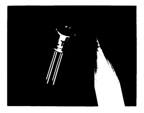
Model 423 contains a <u>Lithium Tantalate</u> sensing element. Lithium Tantalate has a low temperature coefficient, low microphony and no degradation over time. Internal Circuit and Pin configuration
