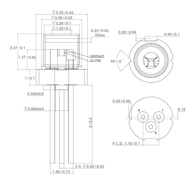
Note : Tolerance is  $\pm 0.05 \text{mm}$  for items without tolerance marking
