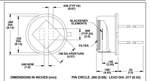
(\*) NOTE: OVERALL HEIGHT DEPENDENT ON THICKNESS OF FILTER AND HEIGHT OF THE CAN. WILL BE EITHER: 0.190" (FOR .010" TO .030" THICK FILTERS) OR 0.250" (FOR .031" TO .090" THICK FILTERS).
