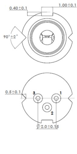
Note : Tolerance is  $\pm 0.05$ mm for items without tolerance marking
