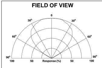
For -3 filter only. For other filters, consider refractive index and thickness.
