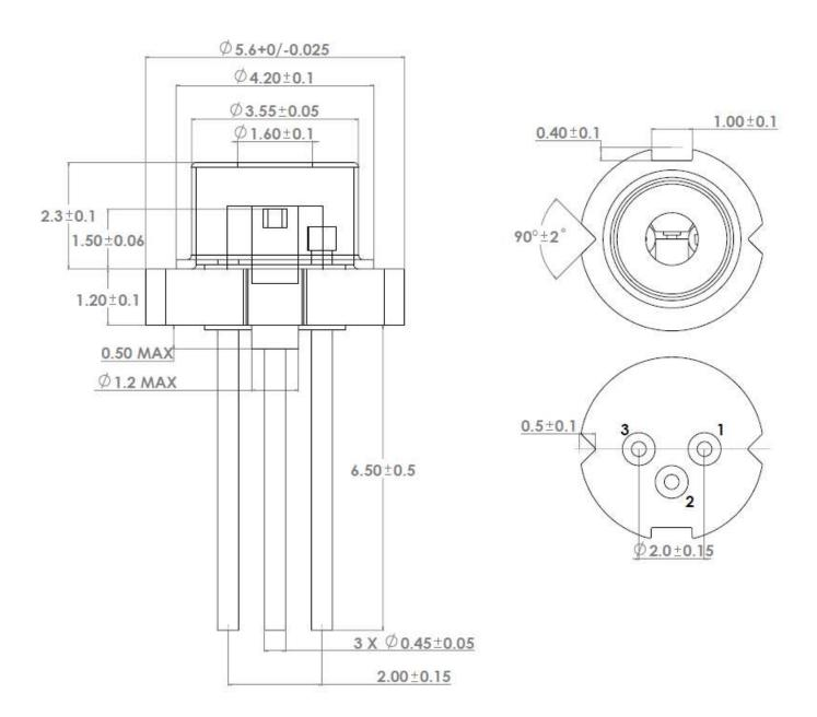
Note: Tolerance is  $\pm 0.05 mm$  for items without tolerance marking
