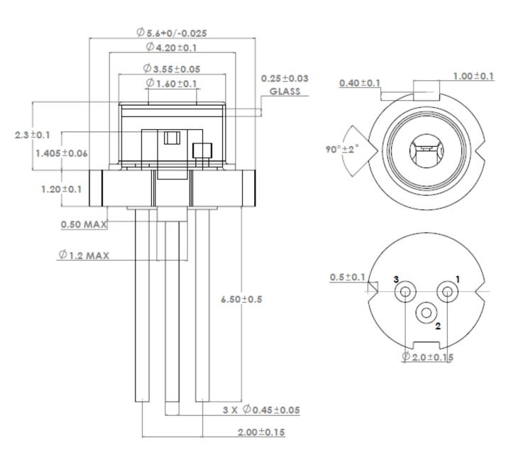
Note : Tolerance is  $\pm 0.05 \text{mm}$  for items without tolerance marking
