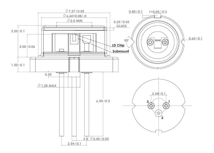
Note : Tolerance is  $\pm 0.05$ mm for items without tolerance marking
