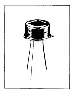
Model 414 consists of two separate sensing elements on a single lithium tantalate crystal and a JFET source follower sealed into a TO-5 transistor housing with optical filter.
