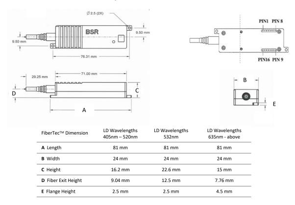
FiberTec™ and FiberDrive™ modules come with 1 meter connectorized fiber pigtail output as standard. Fiber Jacketing options include a 900μm PVC jacket with a bend radius of 13mm or an 3mm Armored metal jacket with Bend radius of 30mm.
