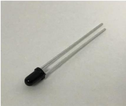
The VTP3420LA is a Si photodiode (PD) mounted in a long T-1 (3mm diameter) plastic package. The package material is infrared transmitting and visible blocking. The PD's sensitivity characteristics make it suitable for smoke detection and infrared detection applications.
