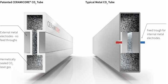
CERAMICORE® CO, eliminate laser gas contamination ensuring stable power, beam quality and longevity.
