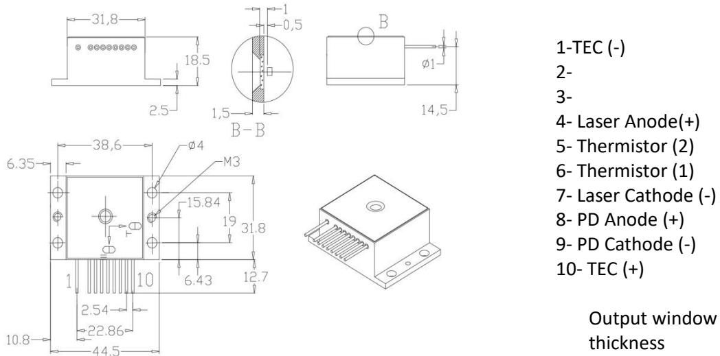
Output window of 0.5 mm in thickness
