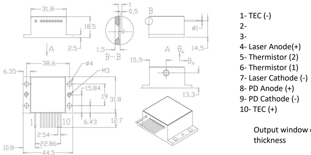
Output window of 0.5 mm in thickness
