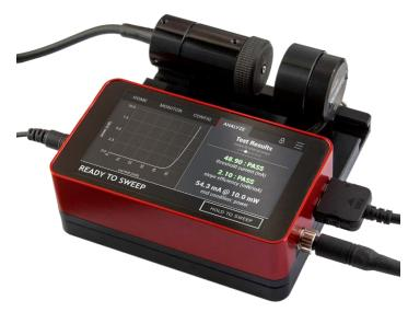
View the results on the modern touchscreen interface or connect the system to your computer to download and process the raw data. The high-performance smart driver automatically detects your diode pinout and can drive the diode in auto-current or auto-power control modes. The integrated TEC controller maintains your diode at its operating temperature ensuring accurate and repeatable measurements.
