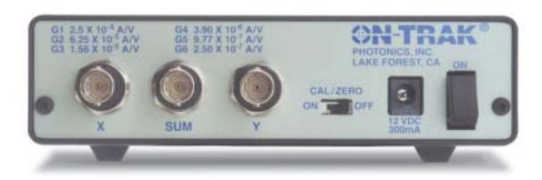
**X Out:** Normalized X axis output (± 10V).
